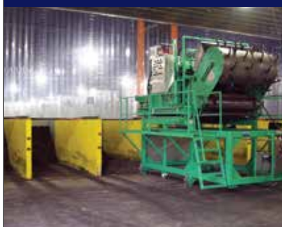
Agitated and Aerated In-vessel type Composting System (ICS)
